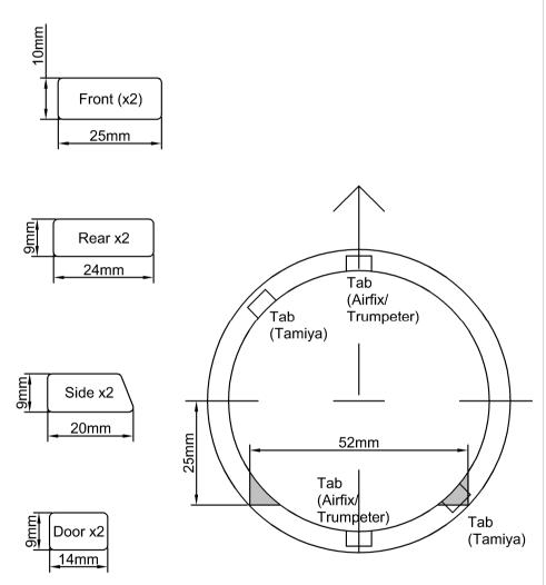
Cut notches in rear corners of turret ring to fit the interior.
